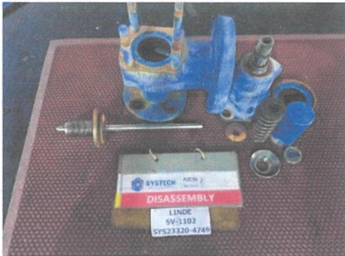
Valve Dis-Assembly
