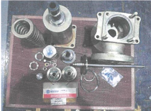
Valve Dis-Assembly
