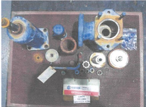
Valve Dis-Assembly
