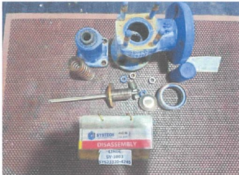
Valve Dis-Assembly
