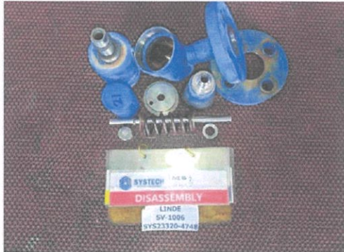
Valve Dis-Assembly
